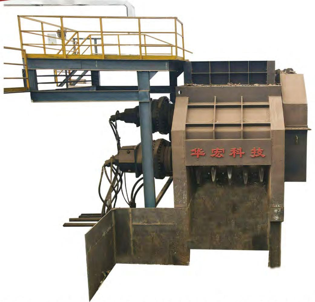
YSJ Series Scrap Metal Pre-shredder are suitable for the pre-shredding treatment of car shells and metal bales (density less than 1.5t/m<sup>3</sup>), torn into small pieces or strips, and then transported to the scrap steel shredder line for final shredding.
