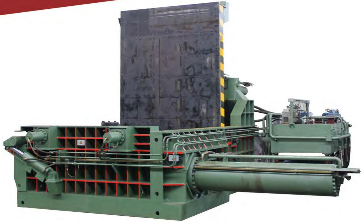
Y81 series of hydraulic scrap balers are applied in thickness less than 6mm steel mills, recycling plants, ferrous & non-ferrous smelting industry to press scrap metal (steel, copper, aluminum, stainless steel, discarded automobiles, etc) into acceptable furnace charges in shapes of cuboids, cylinders & octagons. Suitable for scrap processing and distribution center (base), scrap car dismantling and remanufacturing, steel and nonferrous metals industry etc.
