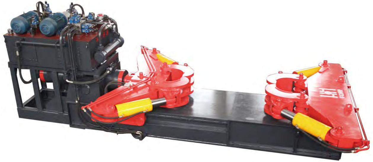
CBJ Horizontal Metal Unpacking Machine are suitable for dismantling scrap cars or scrap bales to facilitate the shredder process of the crushing line or check whether there are impurities in the bales.
