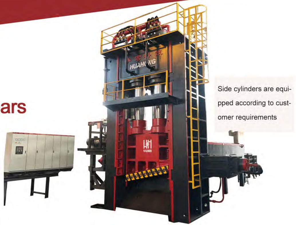
Q91Y Series Heavy-duty Scrap Shears are suitable for cutting light scrap materials, waste car shell, light structural parts, etc. to qualified charge to meet steel smelting requirements.
